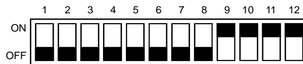
Figure 4-3. Dipswitch Default Setting, Example 1
