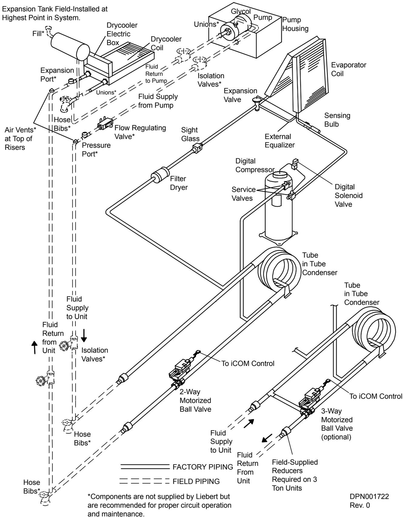
Figure 22 General arrangement—GLYCOOL models with scroll compressor
