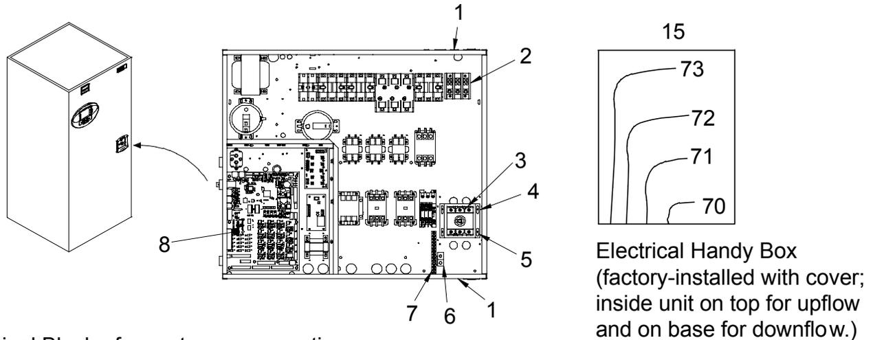
Terminal Block - for customer connections
