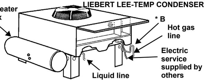
\* B - Inverted traps are to be field-supplied and installed (typ). When installing traps, provide clearance for swing end of access door. Traps are to extend above base of coil by a minimum of 7-1/2" (190 mm)
