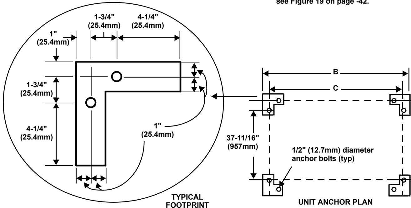
Figure 19 Pump packages—expansion tank
