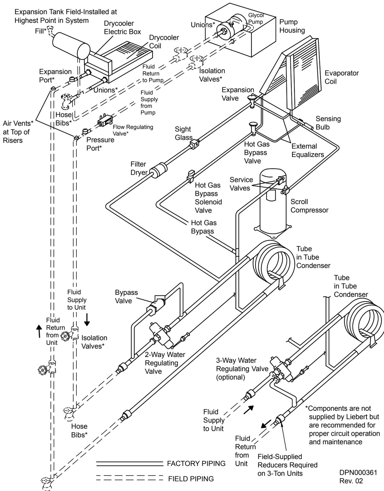
Figure 21 General arrangement—Glycol-cooled models with digital scroll
