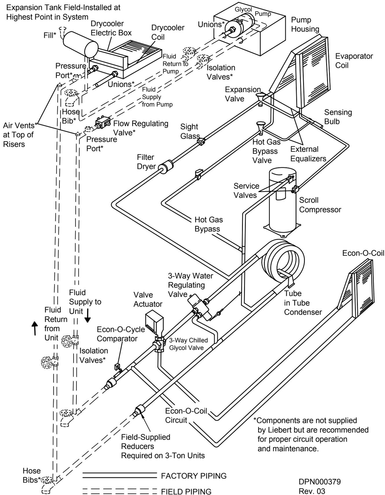
Figure 23 General arrangement—GLYCOOL models with digital scroll compressor
