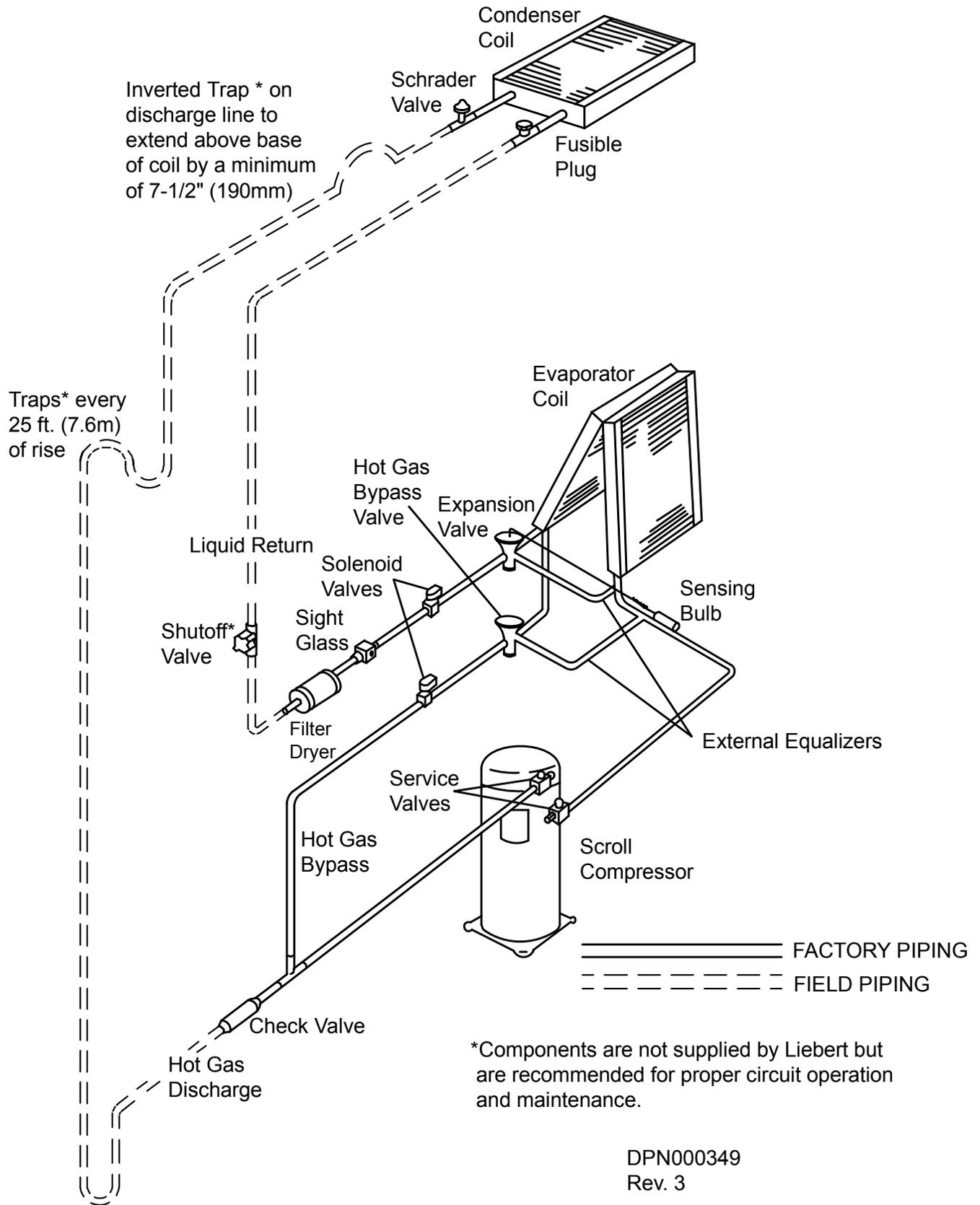
Figure 12 General arrangement—Air-cooled models with digital scroll and fan speed control
