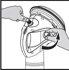
■ **NOTE:** Heater is designed to be lit with the valve fully open until it reaches full output. Observe heat build up for a few minutes to ensure heater is lit. If heater fails to develop substantial heat, turn heater "OFF" and repeat lighting procedure.
