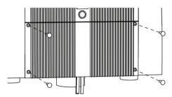
Connect the loudspeakers as required (see *Connecting the loudspeakers*, page 16), then lead all the cables neatly through the slot in the base of the cabinet:
