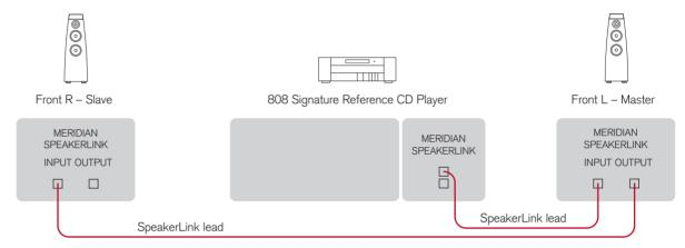
You can create a complete system by connecting a pair of DSP loudspeakers directly to a digital source. The DSP loudspeakers include volume, balance, and tone controls allowing you to control the system using an MSR+.
