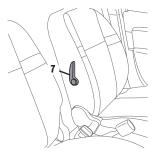
Adjusting the lumbar support on the seat Lower handle 7 to increase the support and lift it to decrease it.
