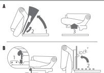
A Removing the seat With the seat folded down (1), gently lower it and lift handle 4 to unlock the front mountings of seat (2). Then guide the seat to the floor (3). Refer to the label located on the back of the seat.
