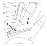
Sliding centre console The centre console slides to allow the length to be adjusted. Lift handle 1 and slide the entire console.
