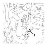
Lift it as far forward as possible (2) until control **4** locks (move the front seat forward if necessary), lower it until it is 10 centimetres from the floor and release it. Check that it is correctly locked. Refer to the label located on the back of the seat.
