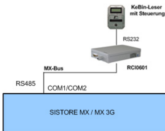
Fig. 24 MX Multi-Channel Box RCI 0601 and access reader – system overview
