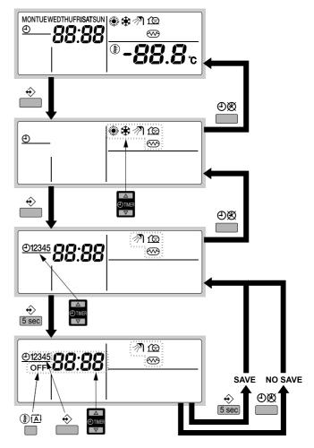
Programming domestic water heating, booster heater or quiet mode is carried out as follows:
