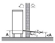
When water is at standstill inside the system, freezing up is very likely to happen and damaging the system in the process.
