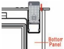
Install the bracket on the bottom of the T7UC in the slots provided.
