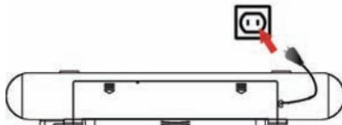
Plug the AC power supply cord of T7UC to the grounded AC socket.
