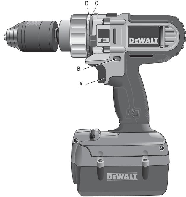
To select reverse, depress the forward/reverse control button on the left side of the tool. The center position of the control button locks the tool in the off position. When changing the position of the control button, be sure the trigger is released.
