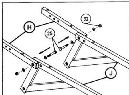
Note 4: Install both bolts (25) as shown (in the direction shown) to connect the two seat braces (H) to the two back braces (J).
