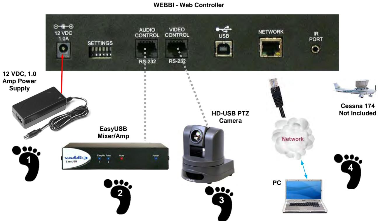
**STEP 1:** Plug 12 VDC, 1.0 Amp power supply included in package into the WEBBi. Power LED on the front panel should light solid blue when powered.
