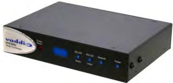
The WEBBi control functions are intended to be used with any device equipped with a web browser and internet access providing an intuitive user interface for control of the room audio and video devices. An embedded web server serves the room's user interface control page to a connected client like a PC, tablet, or smartphone.
