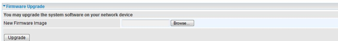
Press the Browse button to select the firmware file and then press Upgrade to start the firmware upgrade process. A progress bar will give indication on the progress of the upgrade. Do not switch off the router or disconnect any cables at this stage.
