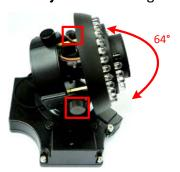
Rotational Adjustment: Using the rotate screw.
