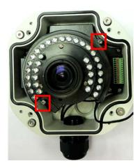
4. Screw the Base Plate to the Wiring Box using the supplied four screws.
