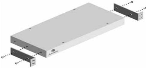
**Figure 2.1: AutoView Switch Horizontal Installation**
