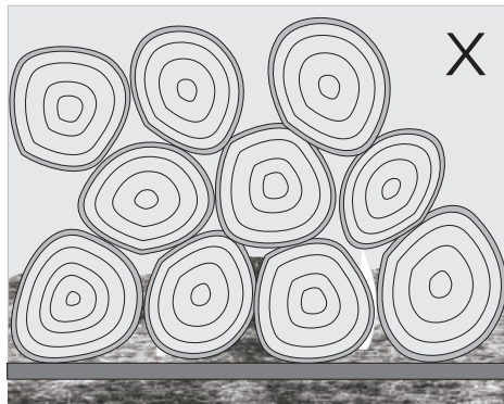
Too many logs. Too little space between the logs.
