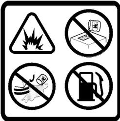
**FLAMMABLE MATERIALS LABEL – LOCATED ON THE UNDERSIDE OF THE RECOVERY TANK.**
