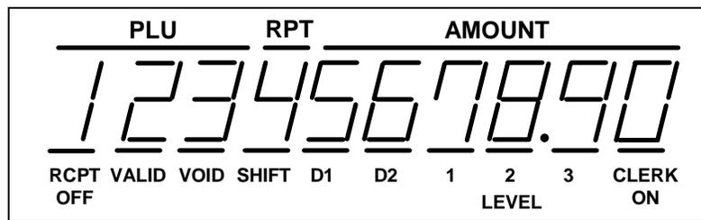
The front display offers supplemental descriptors which appear in the first two display positions (as shown). These descriptors help the operator by supplying additional information while operating the register, and may be accompanied by an error tone.
