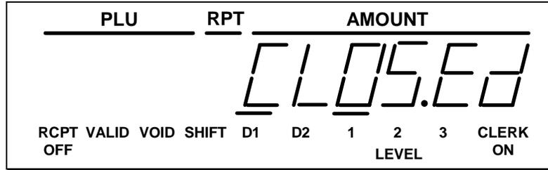
"CL" displayed while in X or Z control lock position indicates that a clerk must be signed on.
