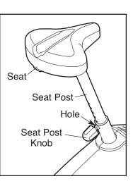
seat post knob. Make sure that the seat post knob is inserted through one of the adjustment holes in the seat post.
