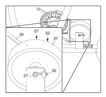
Finally, tighten the 3/8" Nuts (27) and reattach the shields and the pedals.
