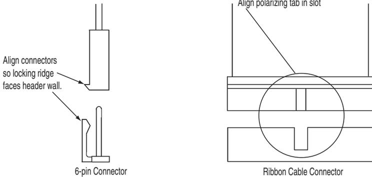
*NOTE: If the 6-pin connector is installed backwards, the power light on this module (and possibly the entire assembly) will not light when powered up. Correct this by separating the modules and locating the reversed 6-pin connector.*
