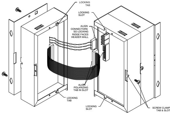
The figure below shows the correct sequence of modules for a maximum assembly. If certain modules are not used, remove them and maintain the order shown for the rest of the modules.
