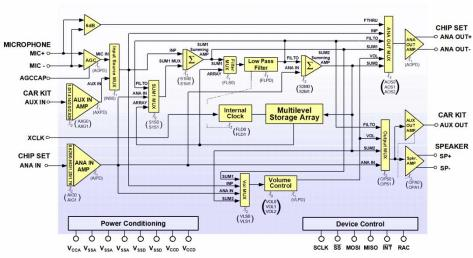
Figure: ISD5008 Block Diagram
