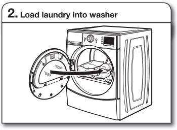
Open the washer door. Place a load of sorted clothes loosely in the washer. Items need to move freely for best cleaning and to reduce wrinkling and tangling. Close the washer door by pushing it firmly until the latch clicks.
