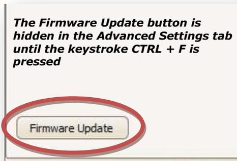
Press the Firmware Update button. The update should take about a minute, and then the controller will reboot.
