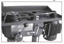
2. Lever the motor, on its bracket, away from the head, by turning lever B - Fig.11, anticlockwise so that tension is applied to the belts.
