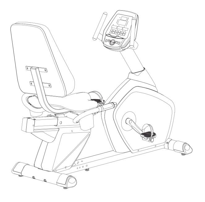
Attach the front stabilizer (B) to the main frame (A1). Line up the mounting holes and secure them with bolts (N7), spring washer (N2) and washer (N3)
