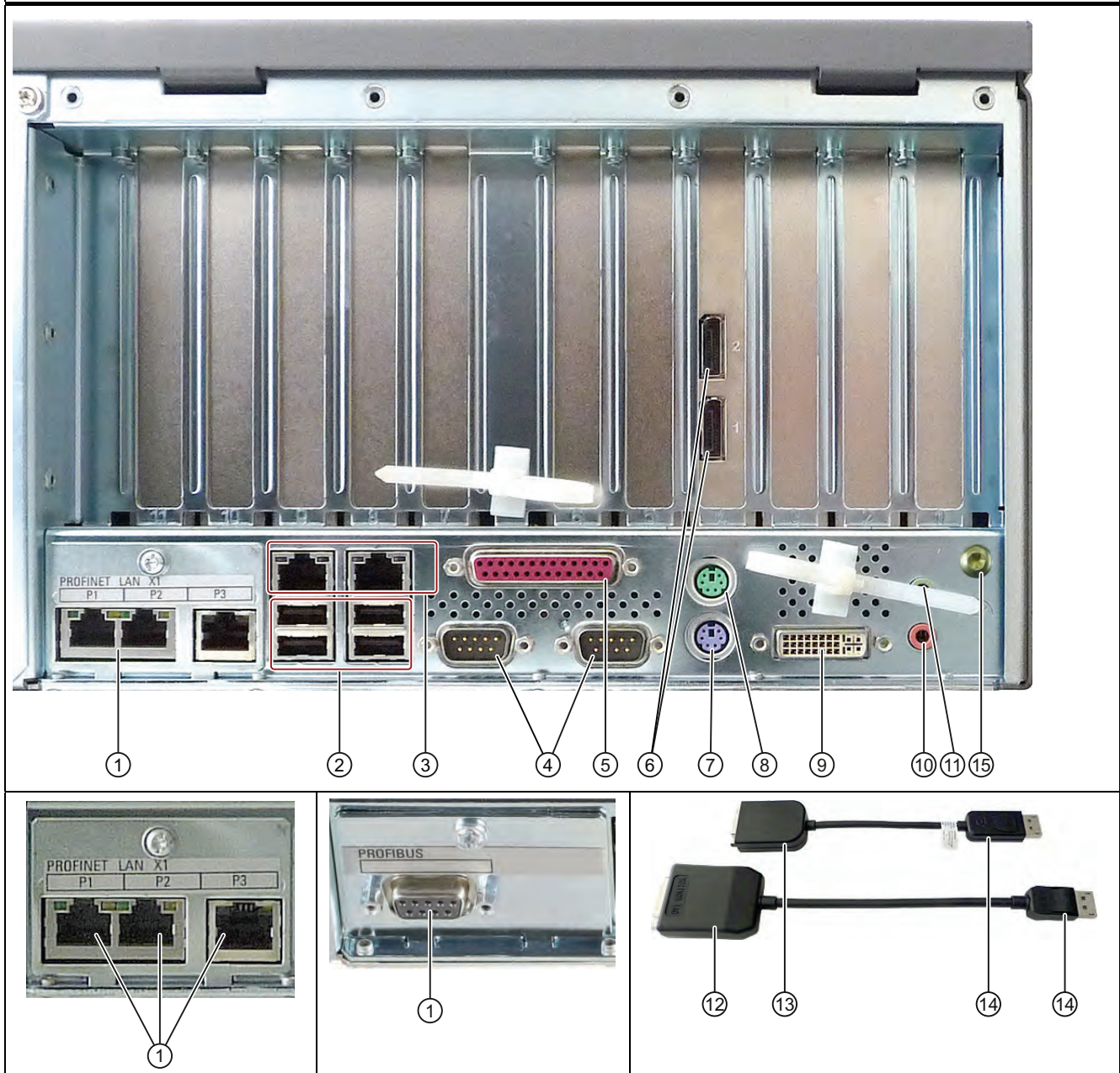
Layout of the interfaces on the rear of the device
