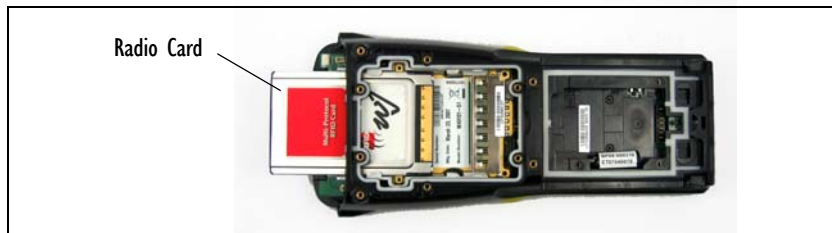
Figure 4 Inserting The Radio Card
