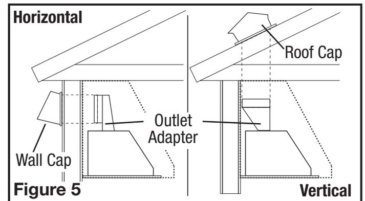
**NOTE:** For models using the B300, B500, or B600 blowers, a minimum of 6" diameter outlet adapter & ducting is required to achieve the proper air flow. The B900 requires a minimum 8" diameter adapter and ducting, while the B1125 requires a minimum 10" diameter adapter and ducting.
