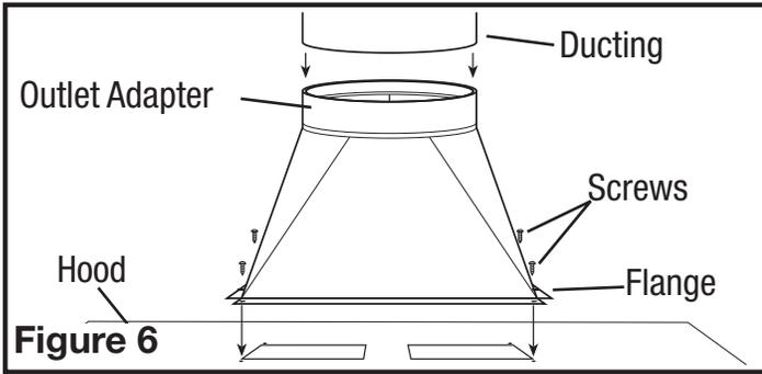
3. When there is access to the top of the unit, connect the ducting to the duct collar and secure in place using tape to seal all joints (Figure 6).
