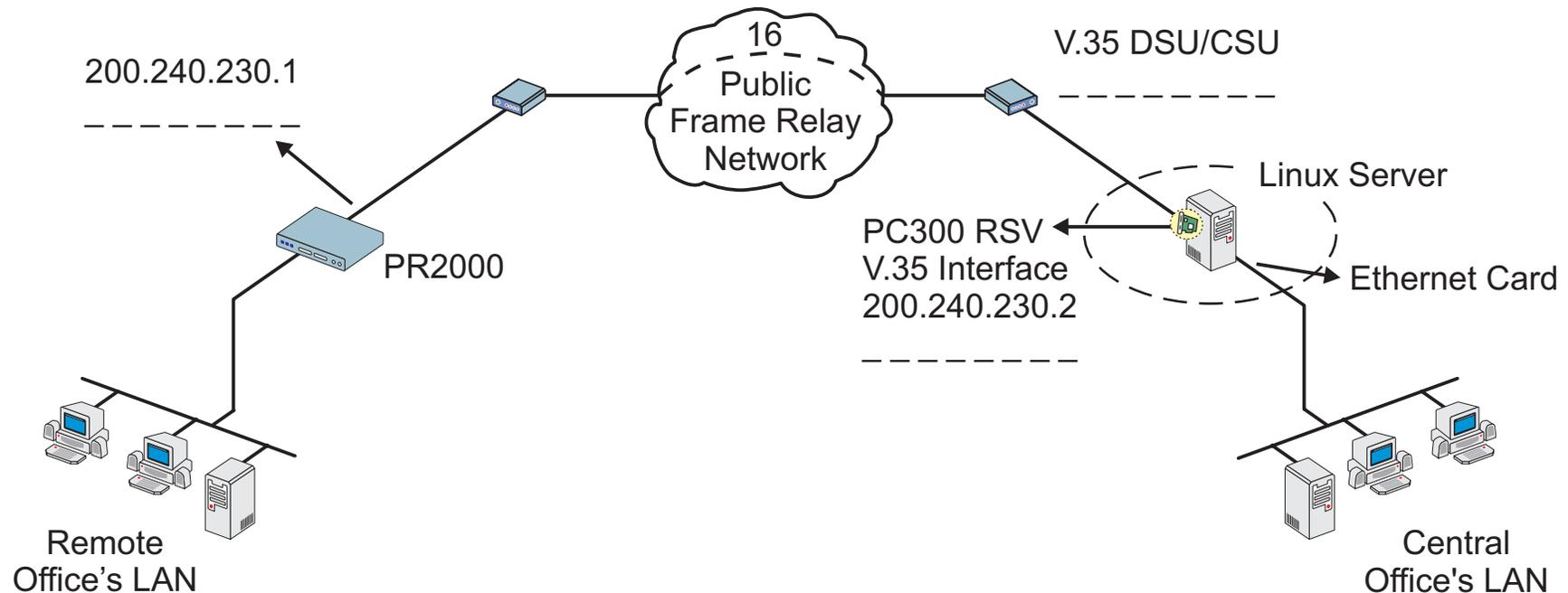
FIGURE 4.2 CENTRAL AND REMOTE OFFICES CONNECTED USING FRAME RELAY
