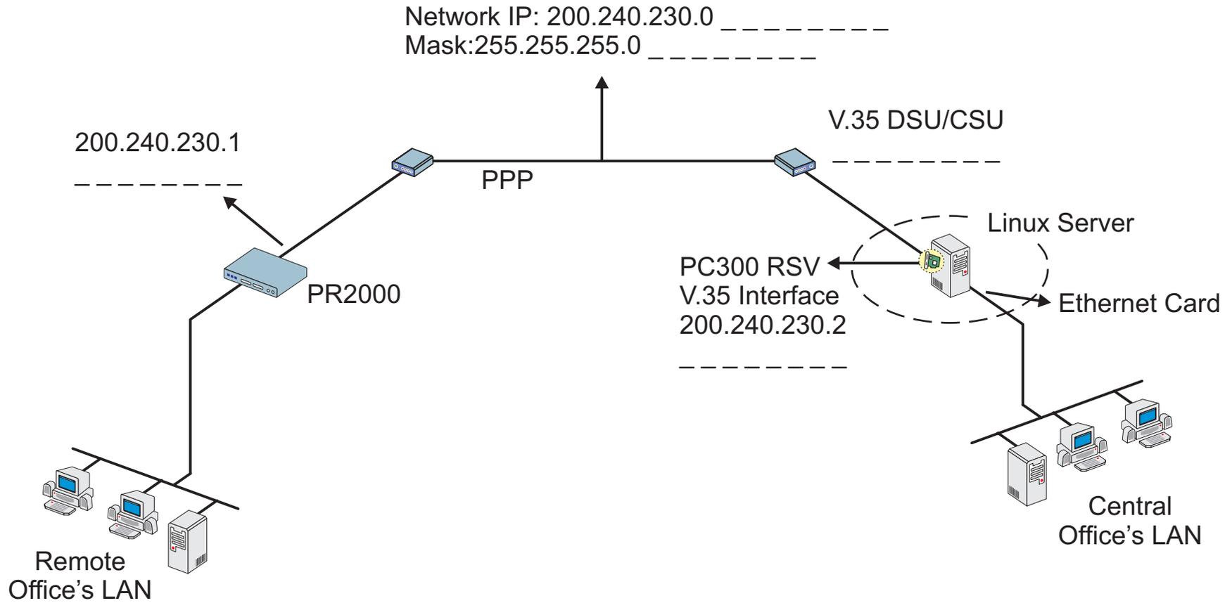
FIGURE 4.1 CENTRAL AND REMOTE OFFICES CONNECTED USING PPP
