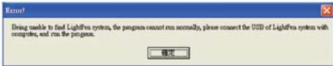
Should the Lightpen icon appear with a red cross in your Toolbar, the USB cable may have been disconnected at computer/projector. Check connections are correct and secure.
