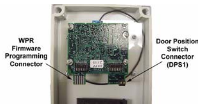
Figure 8-2 – WPR PCB Connectors – WPR Original Version
