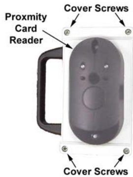
Figure 9-1 – WPR2 with Proximity Reader
