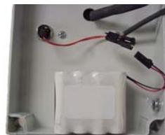
Figure 8-4 – WPR Battery Pack Positioned
