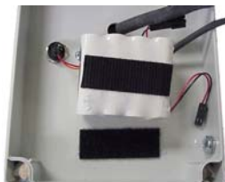
Figure 8-3 – WPR Battery Pack Velcro Strips
