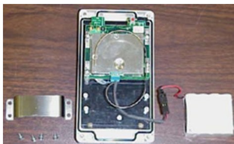
Figure 9-6 - Installing New Battery Pack
