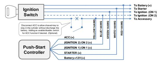
This wiring method also taking into consideration that a shaved-key has been used in ACC position for steering lock bypass. Disconnect the ACC input to the vehicle so shaved-key left in the key cylinder's ACC position does not consume vehicle battery. To retain the full functionality of the key cylinder, add a toggle or latch switch (not included) at the ACC disconnect. This switch allows manual enable / disable the ACC input to the vehicle.
