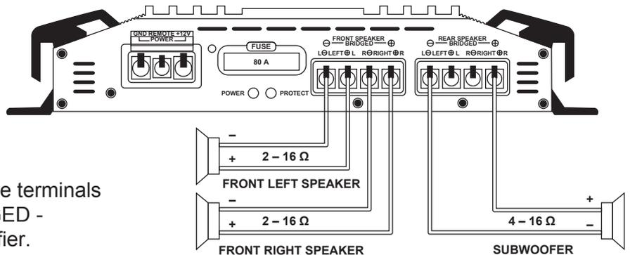
**CAUTION:** Please observe speaker channel and polarity as printed by the speaker terminal block. Incorrect phasing of the speakers results in total loss of bass response.
