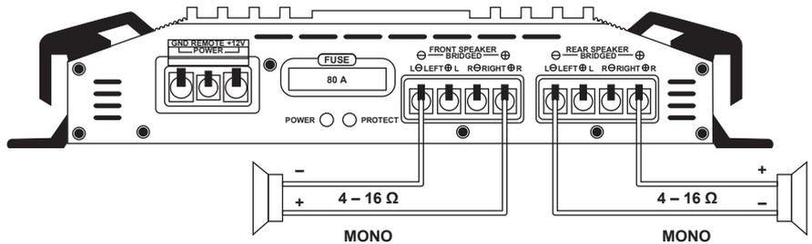
**CAUTION:** Please observe speaker channel and polarity as printed by the speaker terminal block. Incorrect phasing of the speakers results in total loss of bass response.
