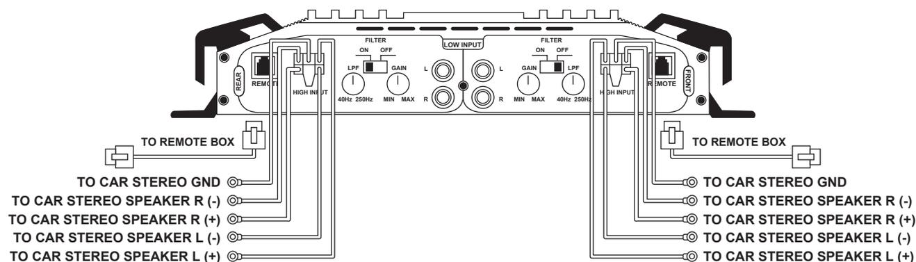
**CAUTION:** Do not wire high and low inputs at the same time. This will result in damage to the amplifier and other units in the set up.
