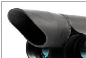
If the HUD image becomes RED after removing sun shield, the available light is too bright and the sun shield should be re-attached.
