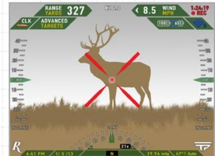
9. When your point of aim and the tag are aligned within the kill zone, the X reticle will turn red indicating the optimal time to fire.
