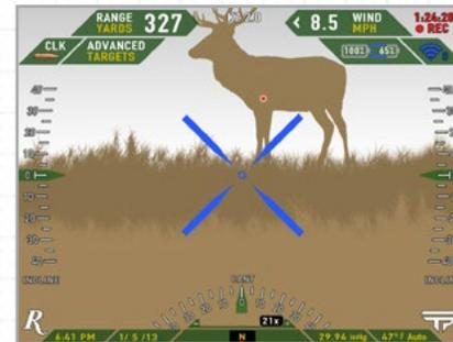
6. When the Tag button is released, a tag is placed on the target and the blue reticle will offset to indicate the actual point of impact for the round based on the ballistic solution for all factors measured by the Remington 2020 and user-input wind.
