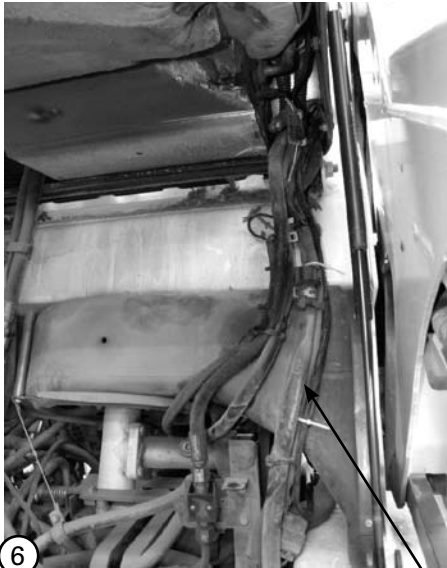
Harness follows existing cab harness
