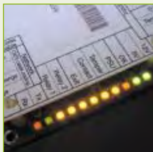
Diagnostic LED's aid installation
