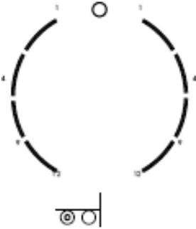
Switch controlling the left, front hot plate.
