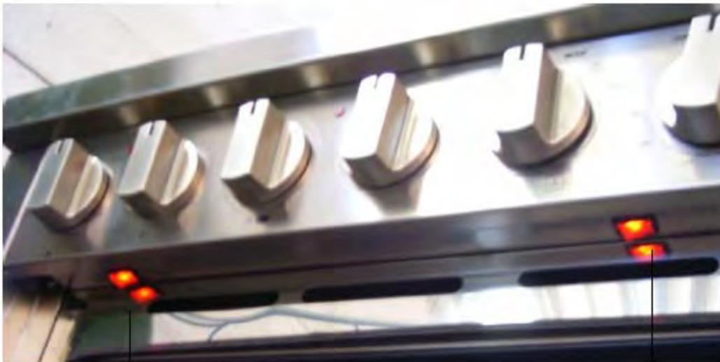
This switch controls the warming element in the oven (200 Watt)
