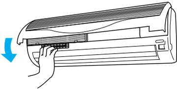
**2** Blow off the dust from the filter with fresh air or wash the filter under running water.
