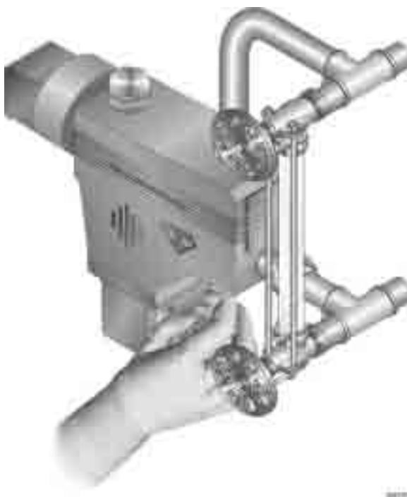
Figure 7 Float type low water cutoff
