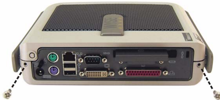
Figure 2-2 Removing the rear screws
