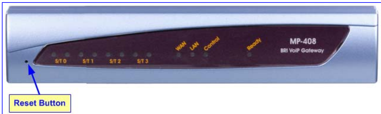
Figure 2-1: MediaPack Front Panel
