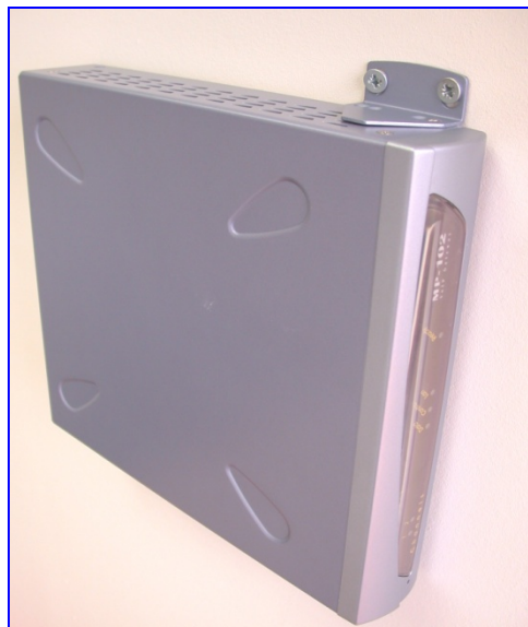
Figure 3-3: MediaPack Wall Mounting
