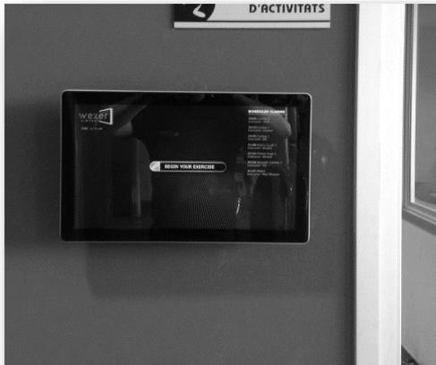
*Installation with a hole drilled in drywall behind the player and the wires hidden in the wall*
