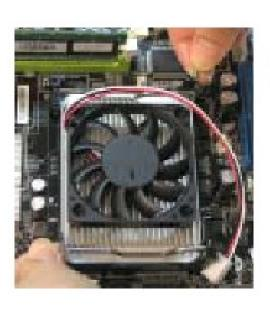
7 . Connect the fan power cable from the mounted fan to the 3-pin fan power connector on the mainboard.
