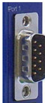
Figure 8. DB-9 Female Serial Port Connector
