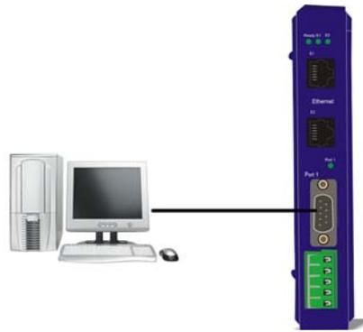
Figure 18. Console Mode Setup
