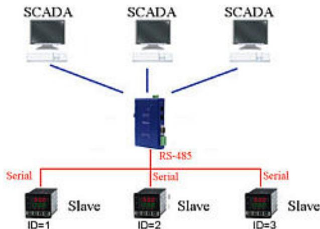
Figure 24. SCADA to Slaves, IDs Configurable
