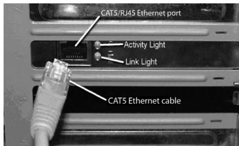
1. Plug your network cable into the device's RJ45 network adapter port.
