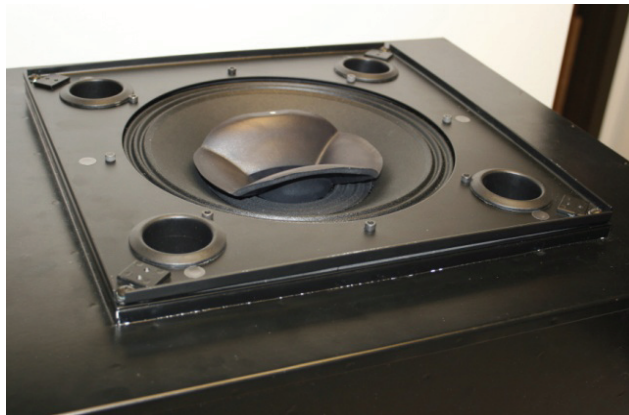
Figure 27: CLOUD12 installed / gasket compressed
