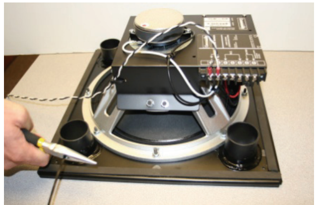
PREPARING TO CUT TIE-WRAP
