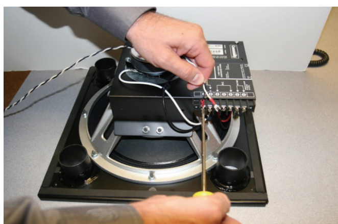
Figure 16: Attaching the loudspeaker cable to the CLOUD12 input panel
