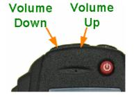
When there is no signal a beep will be emitted at each button press to indicate the volume level. During a call the beeps are omitted.
