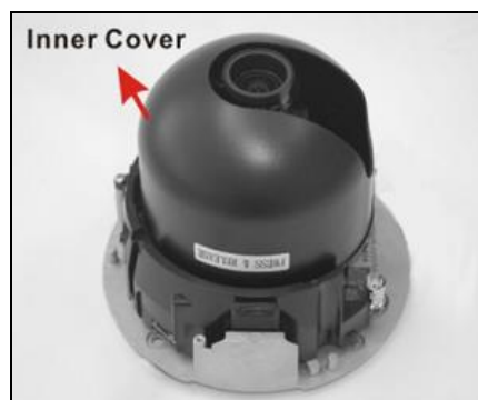
Figure 7: Inner Cover Removal
