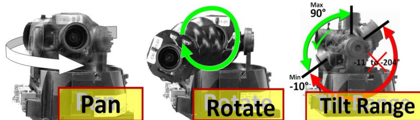
Figure 25: CM-4251 Camera – Pan, Rotate and Tilt Angles
