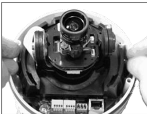
Figure 9: Removing the Camera Module from the Base Plate
