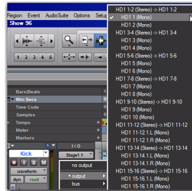
Assigning a Pro Tools track output to a VENUE Stage input channel for Virtual Soundcheck (HDx shown)
