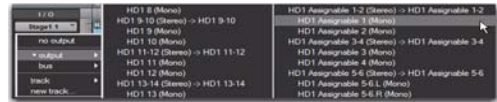
Assigning a Pro Tools track output to a VENUE assignable input (HDx shown)
