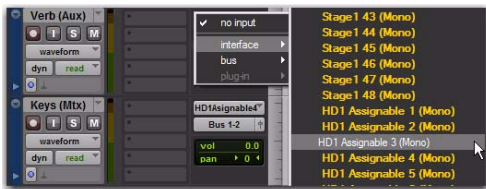
Assigning an HDx assignable output to a Pro Tools track input in the Edit window
