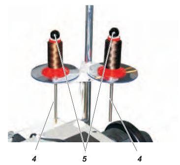
The structure and position of the reel stand 3 can be seen in the illustration.
