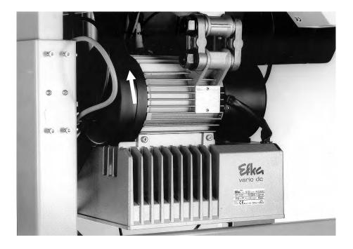
The belt pulley must rotate in the direction of the arrow.
