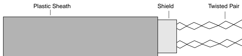
Figure 4-2. Shielded Twisted Pair Cable
